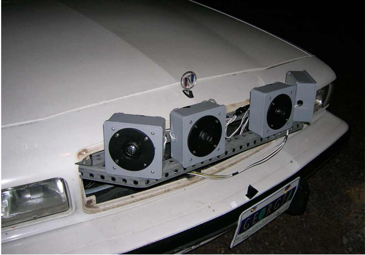
Figure 2.1. Test vehicle equipped with sound-emitting equipment used for observations of behavior of free-ranging white-tailed deer in response to sound treatments at Berry College Campus and Wildlife Refuge, Mount Berry, Georgia, 2006.
