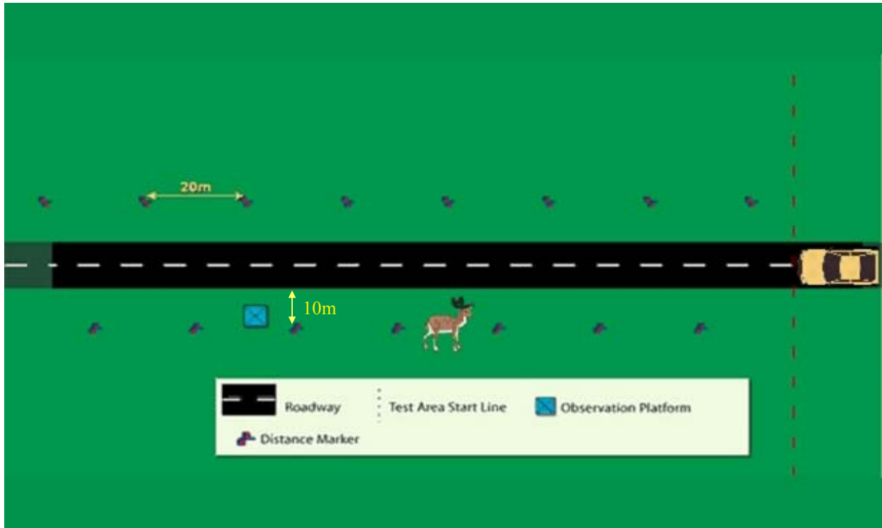
Figure 2.2. Depiction of an experimental roadway section established for testing vehicle-mounted sound deterrents on white-tailed deer roadway behavior on Berry College Campus and Wildlife Refuge, Mount Berry, Georgia, USA, 2006.
